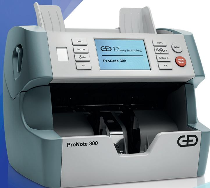
ProNote 300 value counter is particularly suitable for bank branches, currency exchange companies and retailers. In all these areas, the system impresses especially due to its flexible application options. The device is not only able to count banknotes in any currency and verify them according to numerous security features, it can also simultaneously determine the value of processed banknotes.
