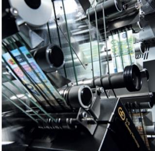
Above: The transport section is designed for high volumes and speed. The integrated NotaScan InOne Sensor provides all the security and reliability that commercial cash centers need to operate, and to fulfill central bank frameworks.
